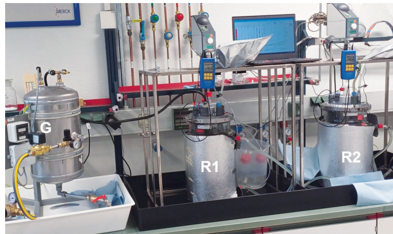
The laboratory biogas plant consists of a gas dosing device (G), a reactor that is supplied with hydrogen and synthesis gas (R1) and the reference reactor (R2) without gas addition.
